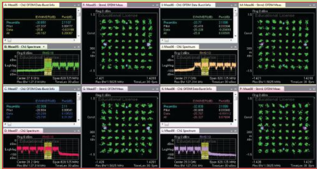
▲ Fig. 7 Measured 8-CCA results for the EMB chip at 28 GHz.
